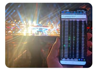
CHT collected a wide array of mobile network performance KPIs, including signal strength, signal quality, signal-to-noise ratio, and download and upload speeds, which gave clear insights into the attendee user experience, compared to other operators.
